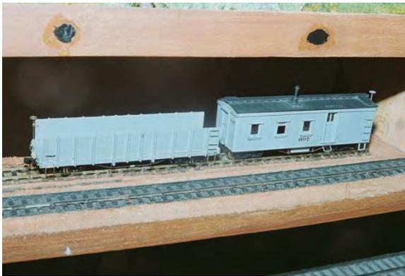
*Photo 3* – Tail end of the new siding on the narrow gauge which is dead level, the mainline track in front is on a 1.6% grade uphill to the next level. Rail is code 70 and code 55.
