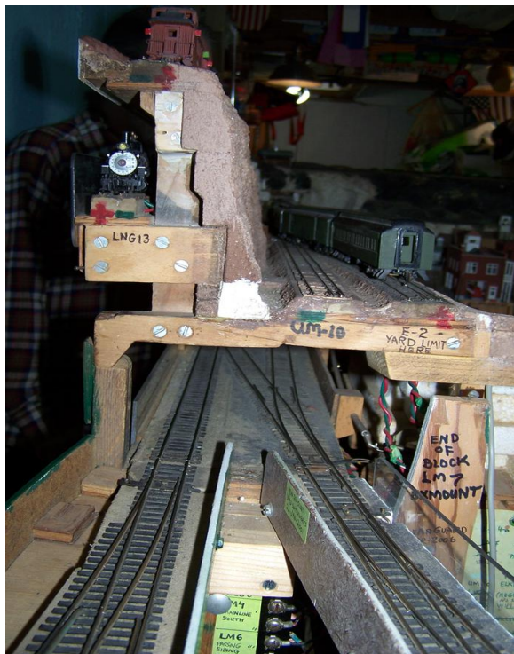
Four tracks cross here: 1) at top is narrow gauge on a flat grade, 2) lower narrow gauge (LNG block 13) with a 1.6% grade, 2
