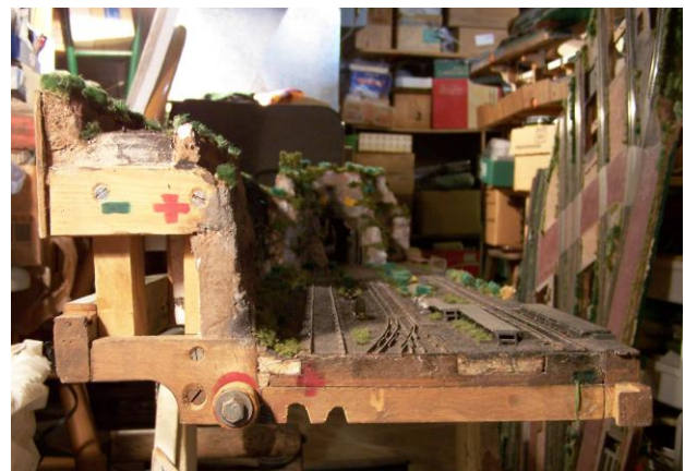
Section MV looking North. The lower dual gauge track is flex-track aligned before completely covering the tunnel, so far, so good. The plywood is suspended from the end plate here, cleats and notches are used to insure alignment of the plywood track base with the next section. Four wires cross here. This bolts to the next section right below the polarity marks. The lift out note is for the Styrofoam scenery which can be removed to clean the track.
