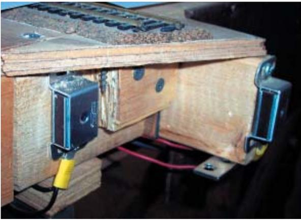
Figure C - Magnets (wired) + L bracket
