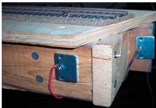
Figure B-Magnet Plates (wired)
