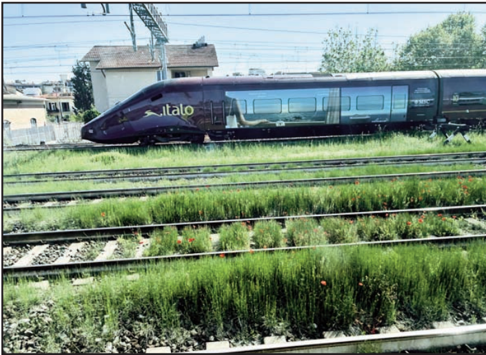
Typical Italo trainset at the Porta Nuova depot in Verona. They ran push-pull, an engine is at each end.
