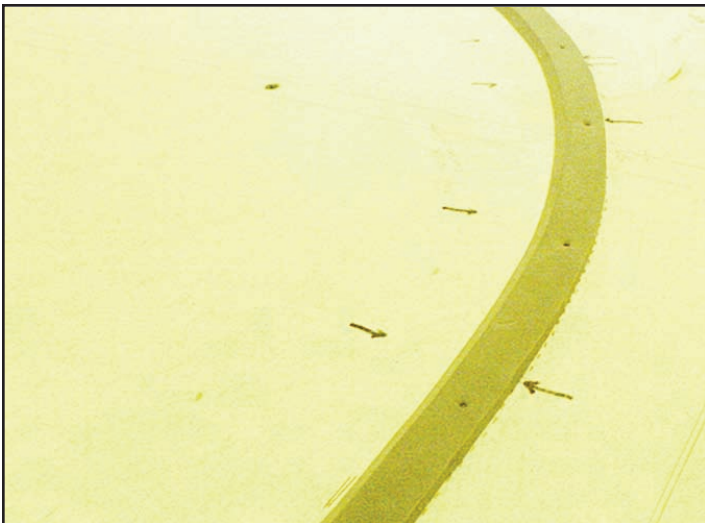
A half piece of foam roadbed cut down the middle and nailed.
